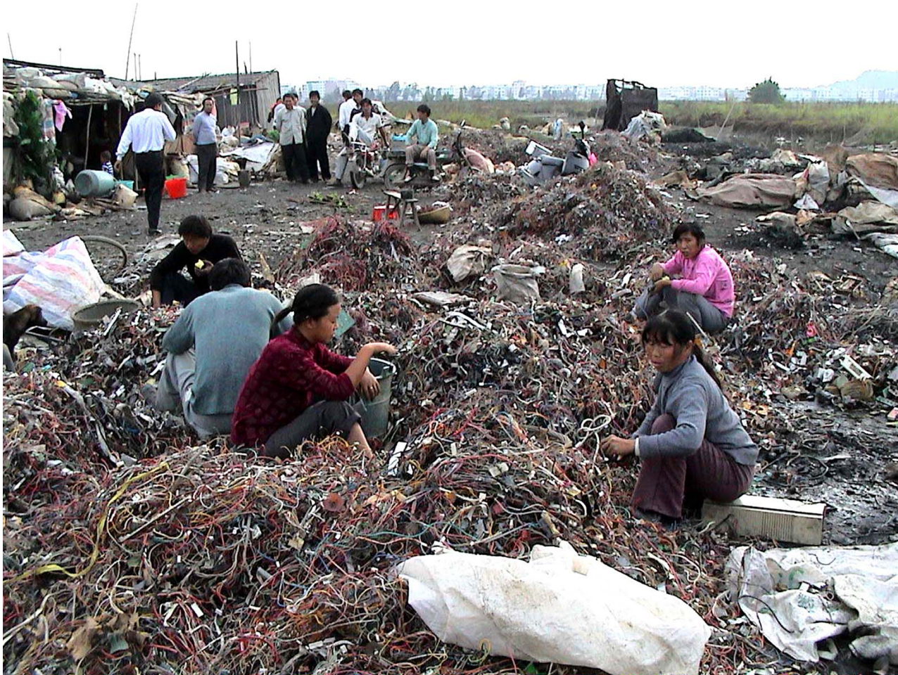
Collecting wires which will later be burned in Guiyu, China. Photo: baselactionnetwork
